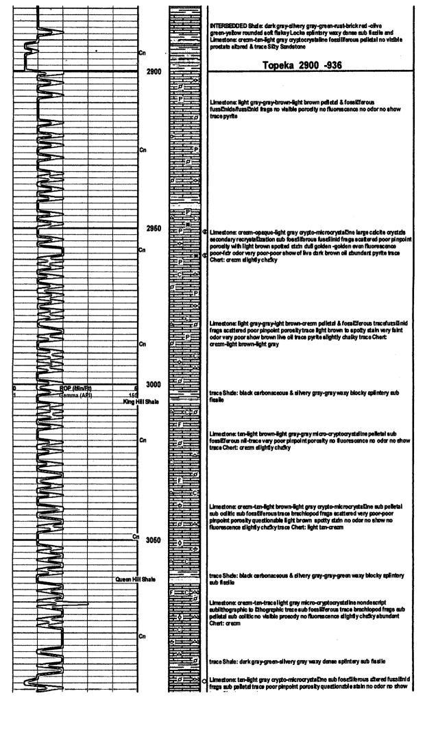
Morgan Ck @ 2907 23:25 6/8/05 Vis 52 Wt 8.6 PV 17 YP 17 WL 7.2 Cake 1/32 PH 11.5 CHL 2,600 ppm Sol 2.15 LCM: 1/2 ppb CMC: \$4,124.00 DMC: \$4,578.00
