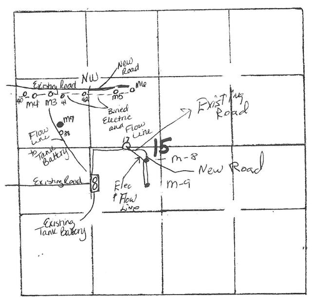
• Proposed Wells - To be completed using existing Flow Lines and Existing Teanly Battery.
