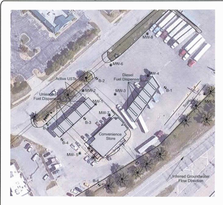
Proposed Soil Boring Location (borings denoted with (G) for hydrologic samples)
