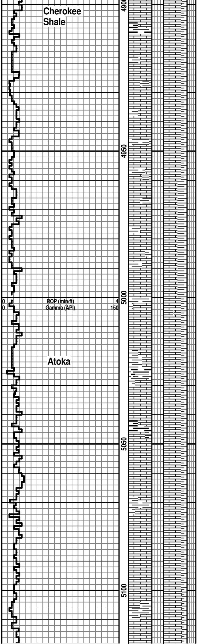
LS:crm tan lt brn ip,vry fn xln fn xln ip,mod hd hd,sl chlky,shly ip,sme calct,tr glauc,sl surc,tr foss frag,sme desm pyr,scat dull yell flor,sme vis frac,no cut
